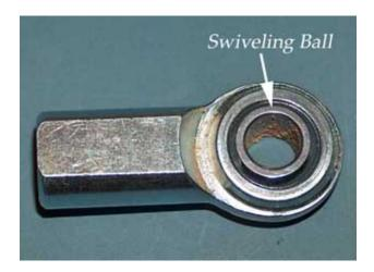
The bearing is a simple hardware store item called a "rod end." The swiveling ball part turns with respect to the rest of object. They come in various sizes. Inside diameter of the ball that I use is 7/16". They come in two genders. This one is female thread up inside from the left end in the picture. It has flat sides with make it easy to clamp. Ones with male threads are not so easy to clamp.
