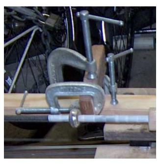
Here is a detail of the picture above showing how I have used a couple of pieces of 1x2 and three C-clamps to position the bearing. The free swiveling ball eases the alignment problem. The rod is padded with a good thickness of masking tape and jammed into the ball, which turns with the rod. A little oil to lubricate it will keep it happy and cool.
